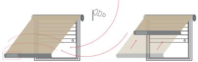
The sensor detects the movement of the awning caused by the wind The awning closes
